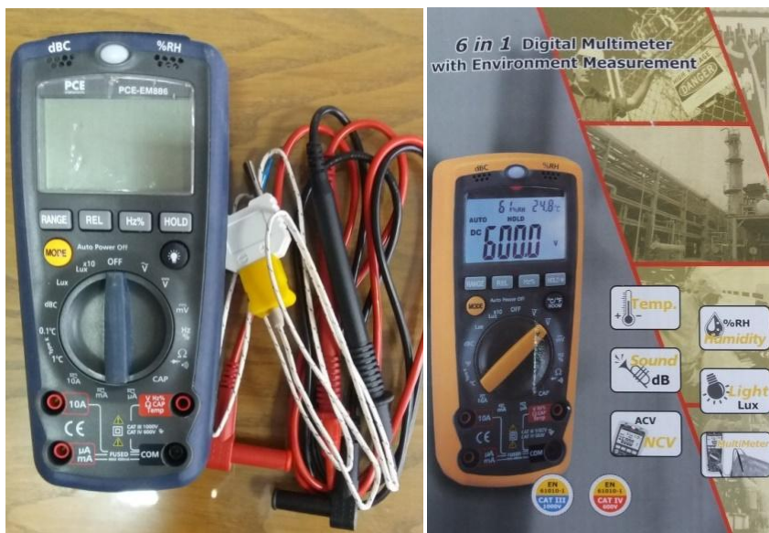
Figure 2 Digital multimeter with environment measurement PCE-EM886
