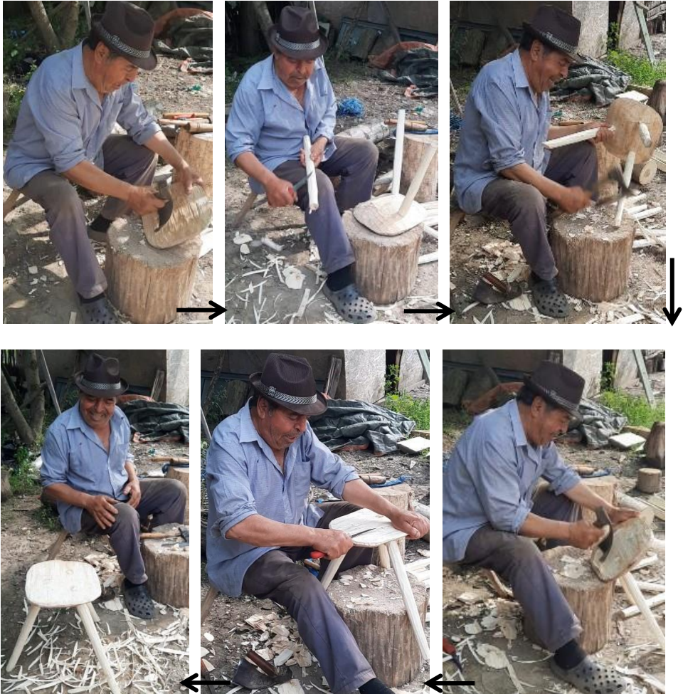
Fig. 2. The stages of making a three-legged chair
