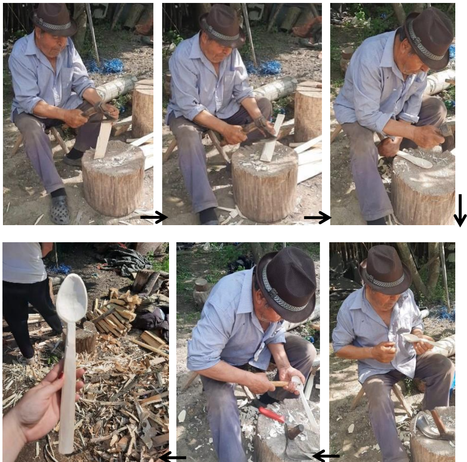
Fig. 3. The steps of making a wooden spoon
