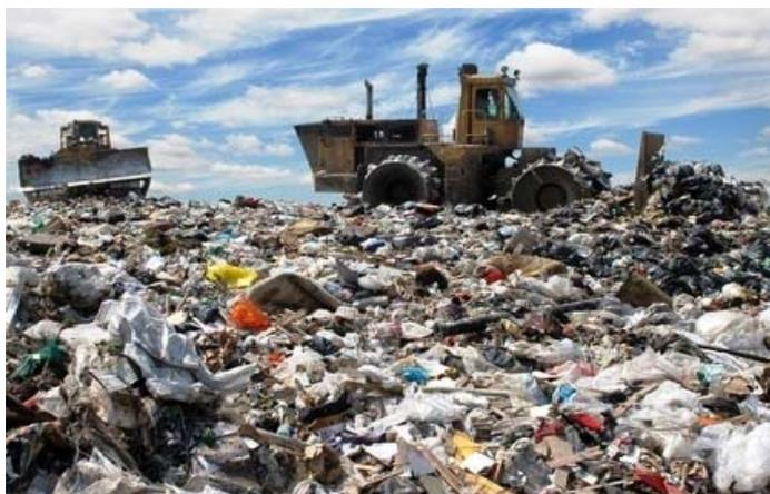
Figure. 3. Bulldozer for depositing of solid communal waste
