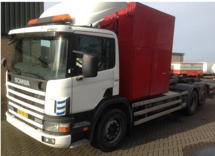
Figure. 2. Vehicle adapted to transportation of refuse containers
