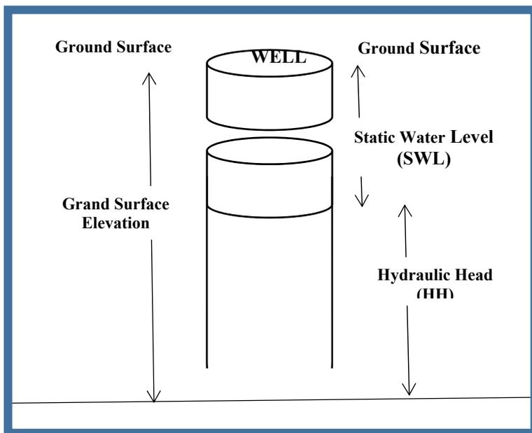
**Fig 2 Schematic Diagram of Measured Variables**
