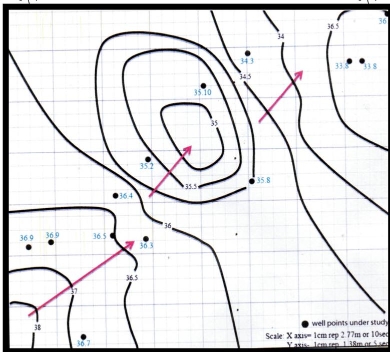
**Fig. 5: Groundwater Flow Direction in the Study**
