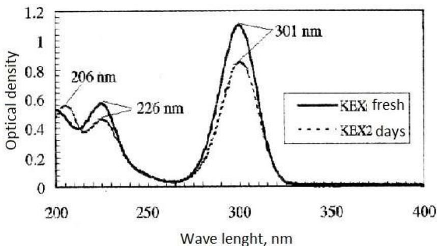
Figure 1, is shown the UV Vis spectra for: ethyl xanthate (ETX-) and carbon disulfide C
