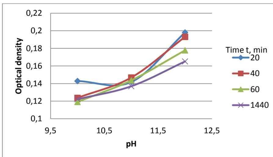
Figure 2. The graphical representation of the concentration of CS<sub>2</sub> in solution as a function of pH and contact time with the mineral chalcopyrite
