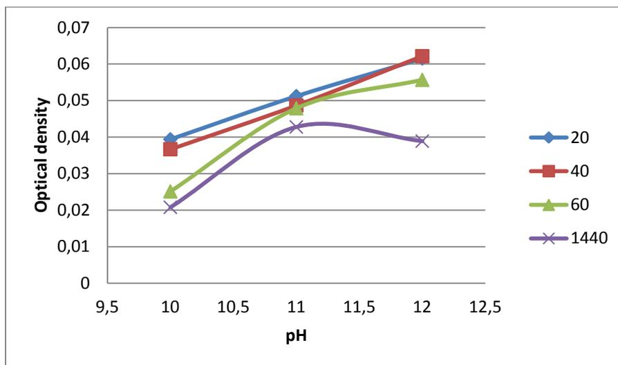
Figure 3. The changes in concentrations of KEX in function of pH and contact time with chalcopyrite
